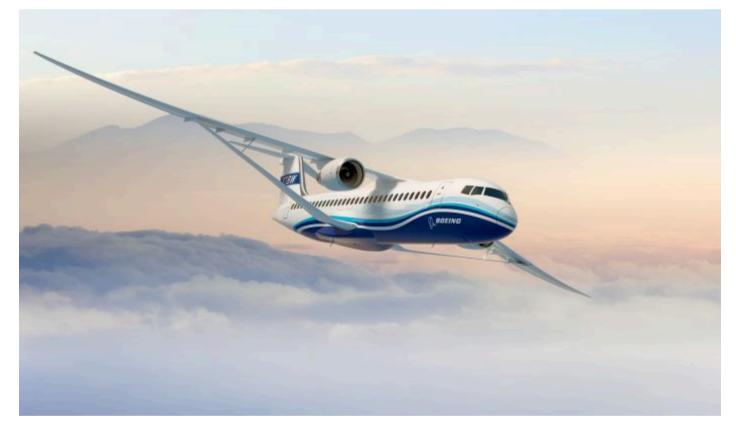
*High-aspect wings, such as this truss braced wing concept from Boeing, could use active flow control technologies to improve performance (Photo: Boeing)*
