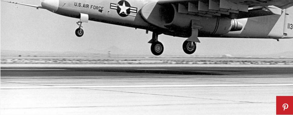
The YA-9 was Northrop's response to the Air Force's late 1960s A-X competition, which called for a simple, rugged, low-cost close-air-support jet designed around a 30mm cannon. Its main competition was a plane you may have heard of: the [Fairchild A-10](#).
