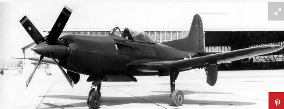
A result of the Navy's continuing interest in jets, the Ryan XF2R-1 Dark Shark was designed to improve over the Bell XP-59 in one key way: Its acceleration would be high enough that the plane could take off from an aircraft carrier. The initial solution was a "composite fighter," a plane that combined a turboprop alongside a turbojet. The Ryan XF2R-1 in particular paired a 1700 horsepower prop with the same GE turbojet used in the XP-59.
