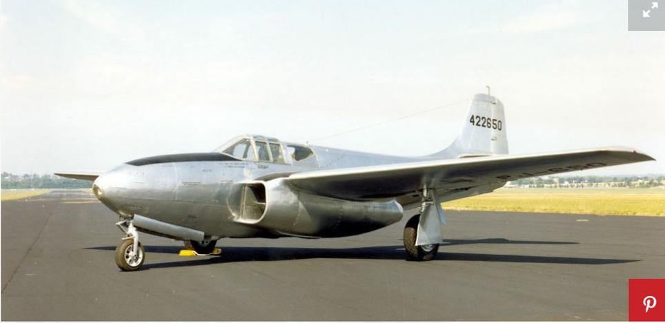
America's first jet fighter plane, the Bell XP-59 Airacomet, was just a bit ahead of its time. Development began in 1941 after American generals saw British inventor Frank Whittle's jet engine during testing in England. Bell Aircraft put two General Electric 1-A turbojets—based on Whittle's design—into a conventional straight-wing monoplane design, one much like propeller-driven fighters of the time.
