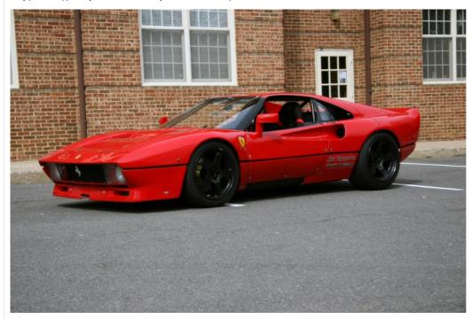
The fiberglass panels are fabricated from real discarded Ferrari 288 molds. However, rather than mounting the conversion panels on a 308 or 328 space-frame, these particular panels enclose a race-ready tube frame chassis. They were combined, as per IMSA GT rules, with the stock-block 308 2.9 liter V8, with suitably modified bottom and top end as well as MOTEC engine management. All that remained of the original 308 was its five-speed manual and its data plate.
