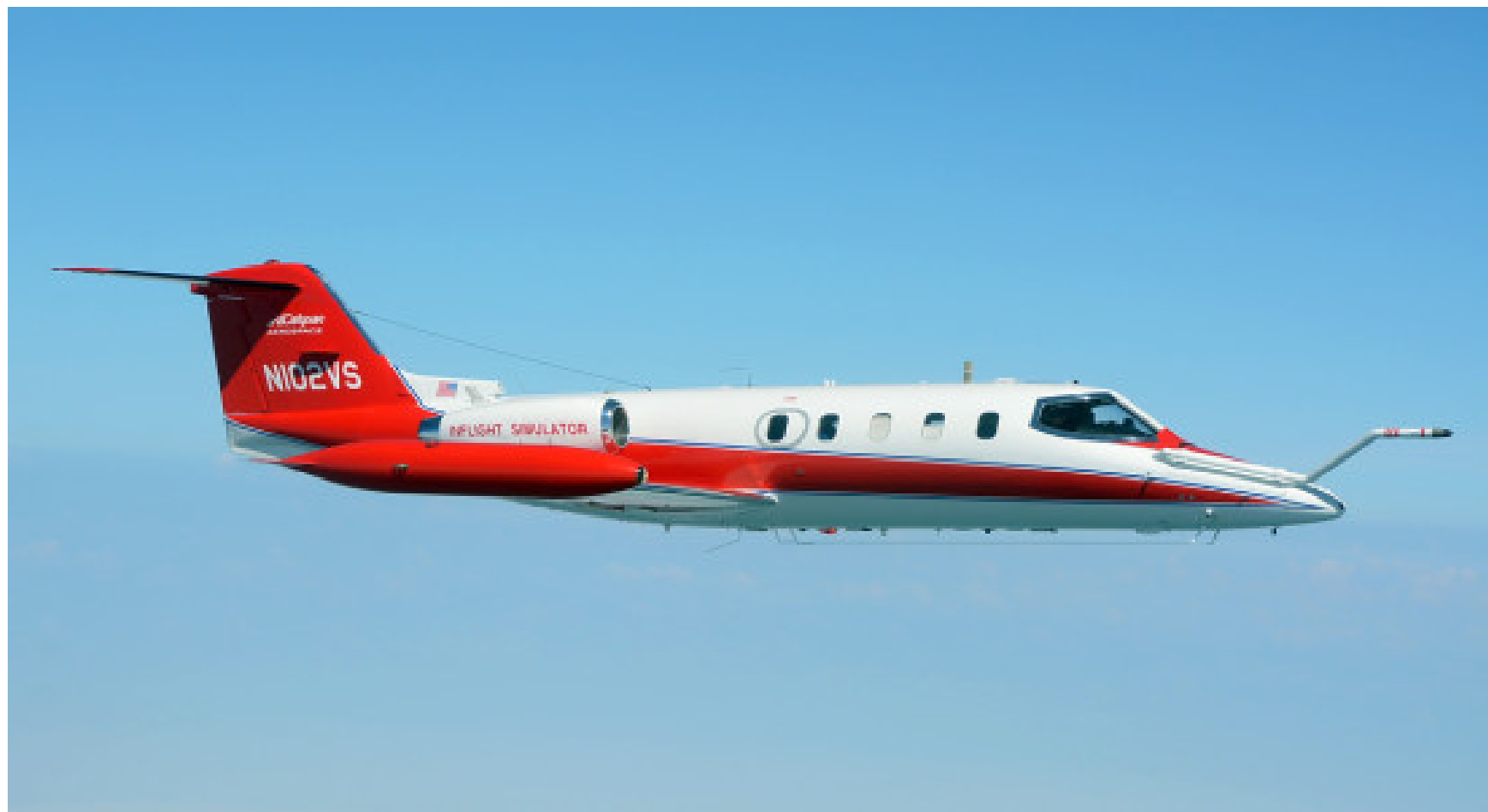
This Calspan Learjet, shown with inert probe in aerial refueling observation position, flies as a surrogate autonomous aircraft. Photo courtesy of CTSi
