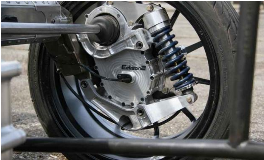
Edison 2's VLC 4.0 is a drivable chassis, featuring an innovative lightweight in-wheel suspension system. Photo by Eric Tegler.
