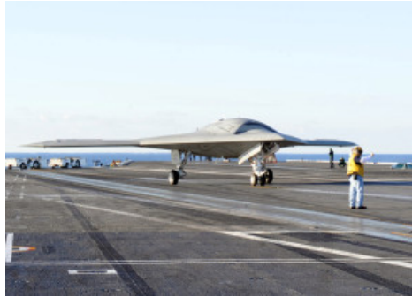
The X-47B demonstrator taxis on the Truman’s flight deck. A crewmember with a remote control unit controls the aircraft under a flight deck director’s orders. U.S. Navy photo by Mass Communication Specialist 2nd Class David R. Finley Jr.
