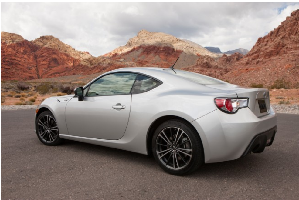
The rear is dominated by a diffuser and a pair of large LED lamps. Photo courtesy of Toyota Motor
