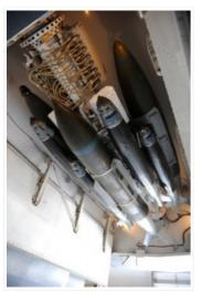
An assortment of 500-pound and 2,000-pound joint direct attack munitions are connected to a multiple ejector rack on a B-1B Lancer March 31, 2011, at a weapons load barn at Dyess Air Force Base, Texas. The 16-carry modified rotary launcher increases the number of 500-pound JDAMs and laser-guided JDAMs carried by a B-1B from 15 to 48, a 320 percent increase in capability. U.S. Air Force photo by Airman 1st Class Shannon Hall
