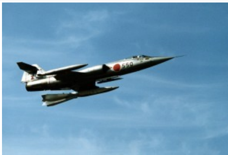
A Lockheed Martin F-104J Starfighter of the Japanese Air Self Defense Force (JASDF) in flight with a target sleeve during a training exercise in 1983. The Japanese F-104J were manufactured by Lockheed Martin but assembled by Mitsubishi. U.S. Air Force photo by Staff Sgt. Steve McGill
