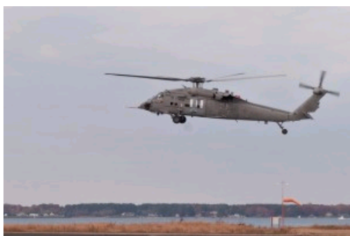
A U.S. Navy MH-60S Sea Hawk helicopter assigned to the Blackjacks of Air Test and Evaluation Squadron (HX) 21 tests a 50/50 Camelina seed-based biofuel blend at Naval Air Station Patuxent River, Md., Nov. 18, 2010. The test demonstrates another step toward the certification of fuels from non-petroleum sources for use in all Navy and Marine Corps aircraft. U.S. Navy photo
