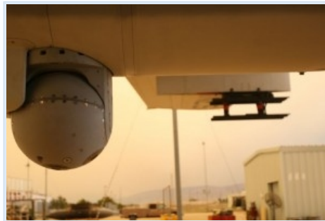
The Harvest Hawk mission kit uses an AN/AAQ-30 Targeting Sight System (left) and an AGM-114P Hellfire II weapons system (launch rails at right) mounted on the left wing of a KC-130J. A fire control operator at a fire control station located in the rear of the aircraft monitors these systems. Official U.S. Marine Corps photo by Cpl. Christopher O'Quin.
